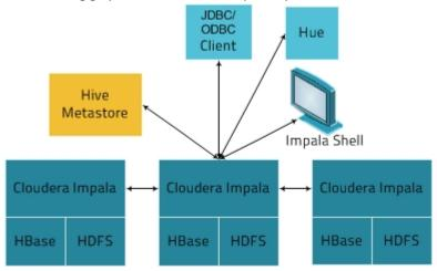
The Impala solution is composed of the following components:
