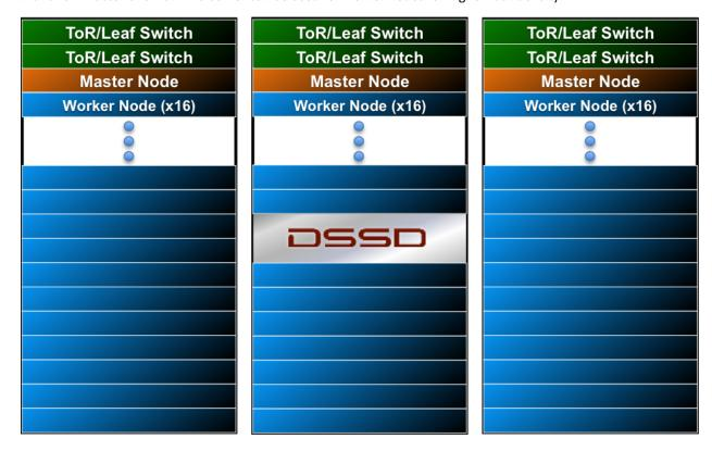
In order to scale both storage capacity as well as compute capacity, add more DSSD D5 appliances and/or worker nodes. Follow the physical layout diagram shown above as a guideline for resource augmentation.
