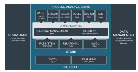
Figure 1: Cloudera Enterprise - Making Hadoop fast, easy and secure
