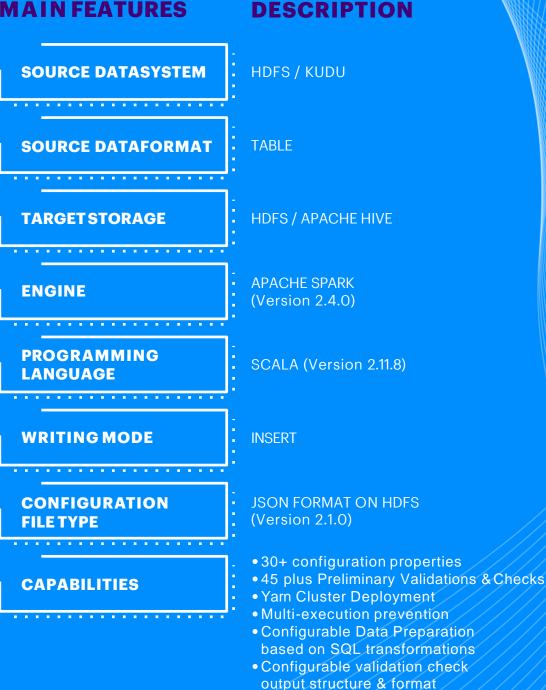
ABIS-T2, the «compactor», consumes files from HDFS to resolve the large number of small files within HDFS locations . It uses defined thresholds to understand which file should be compacted and it stores results into defined Hive tables.
