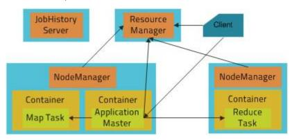
The new architecture has its advantages. First, by breaking up the JobTracker into a few different services, it avoids many of the scaling issues faced by MapReduce in Hadoop 1. More importantly, it makes it possible to run frameworks other than MapReduce on a Hadoop cluster. For example, Impala can also run on YARN and <a href="mailto:share resources">share resources</a> with MapReduce.
