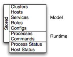
Cloudera Manager models CDH and managed services: their roles, configurations, and inter-dependencies. *Model state* captures what is supposed to run where, and with what configurations. For example, model state captures the fact that a cluster contains 17 hosts, each of which is supposed to run a DataNode. You interact with the model through the Cloudera Manager Admin Console configuration screens and API and operations such as "Add Service".
