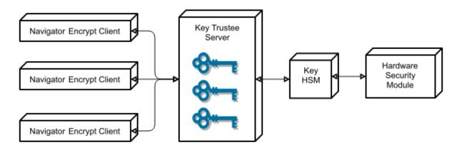
Key Trustee clients include Navigator Encrypt, Key Trustee KMS, and HSM KMS. Encryption keys are created by the client and stored in Key Trustee Server.
