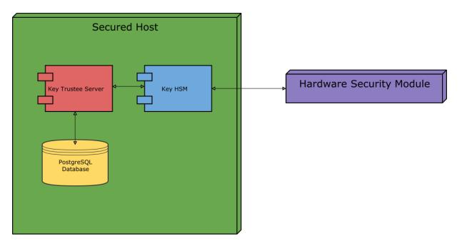
The following diagram displays the recommended architecture for Key HSM:
